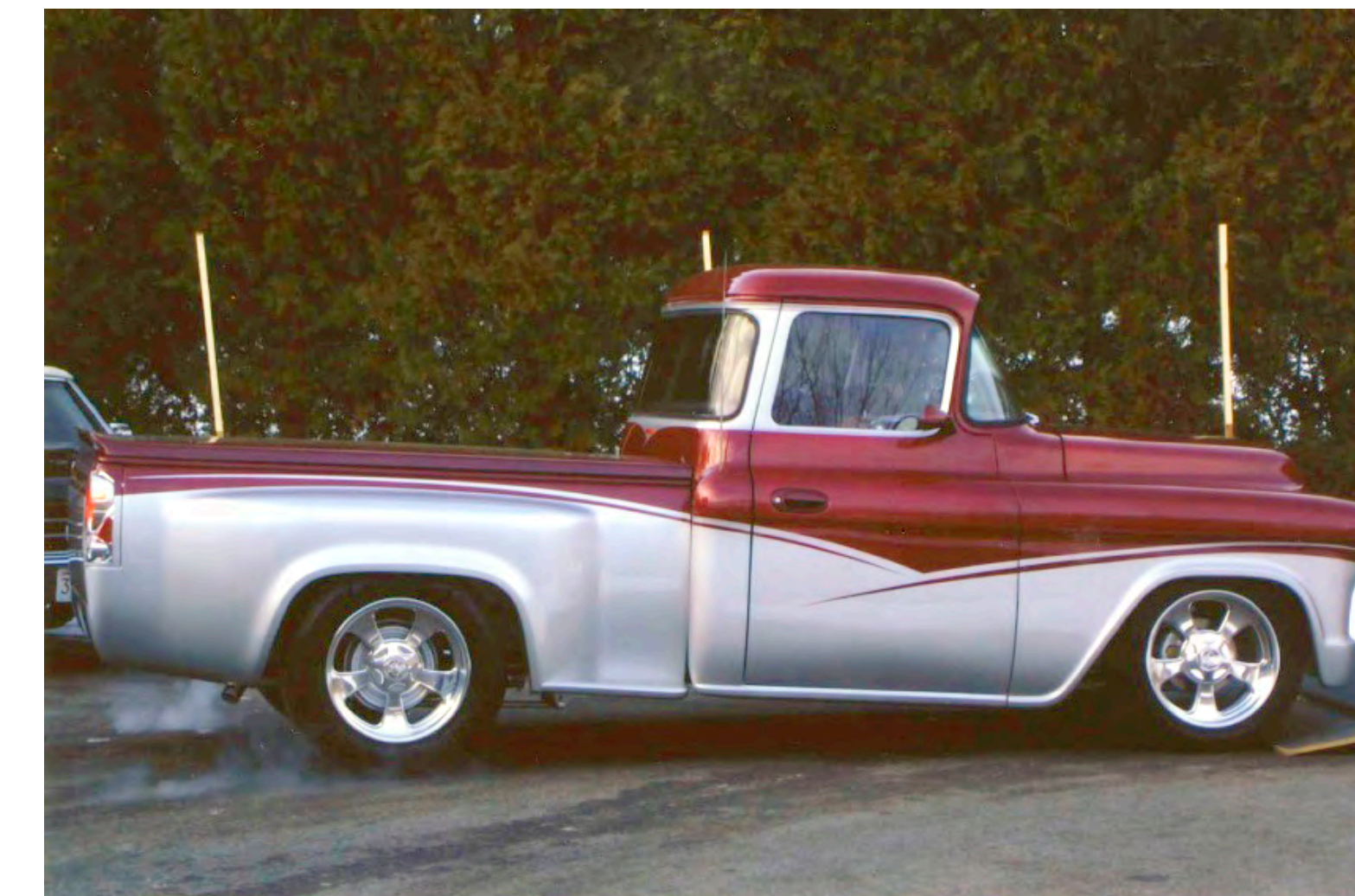
Body with slight forward "rake" created by larger 18" wheels on back
