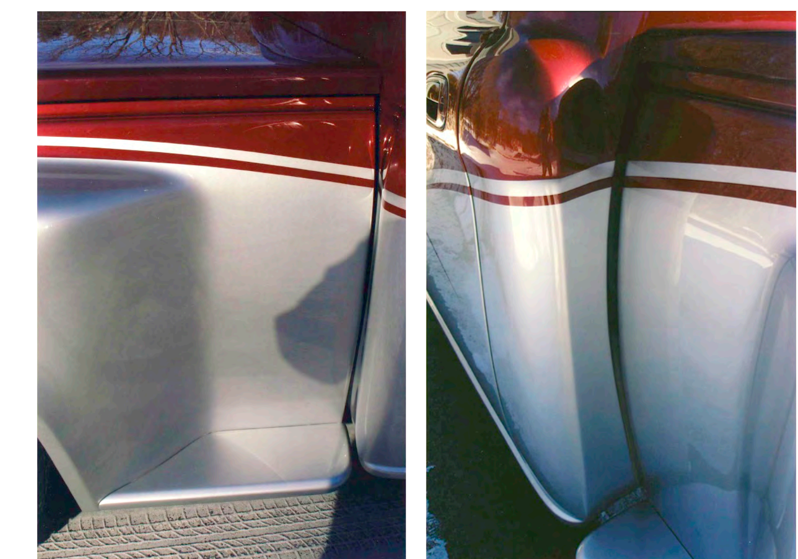
Back of cab has been contoured to shape of bed; new 1955-like "steps" were designed to fit custom fenders
