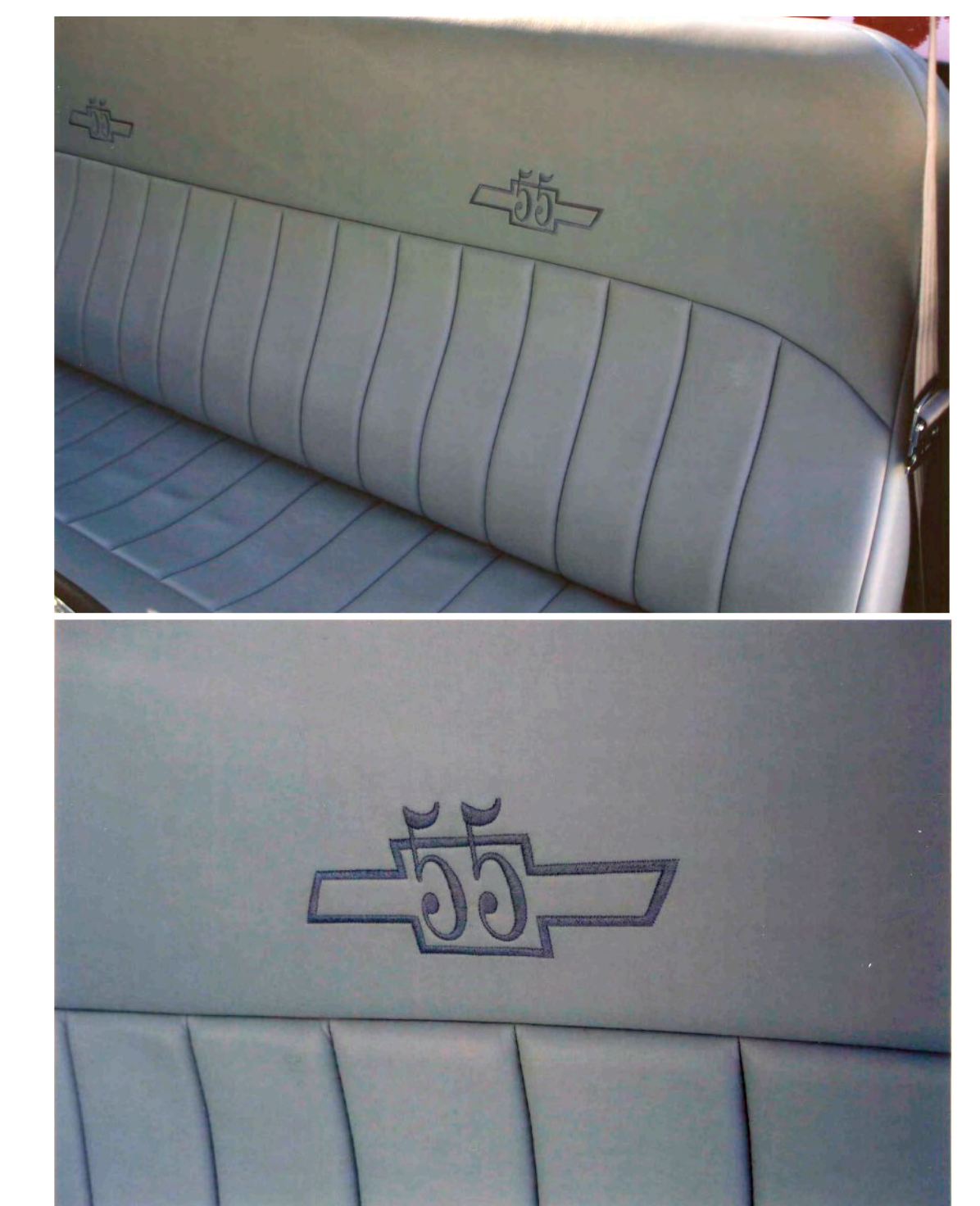
Custom seat with embroidered Chevy "Bow Ties;" inside of cab is completely covered with "ultraleather" with German wool carpet
