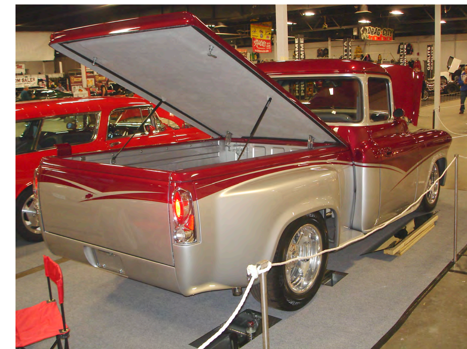
Tonneau cover over truck bed has slight "spoiler;" underside of tonneau cover is carpeted
