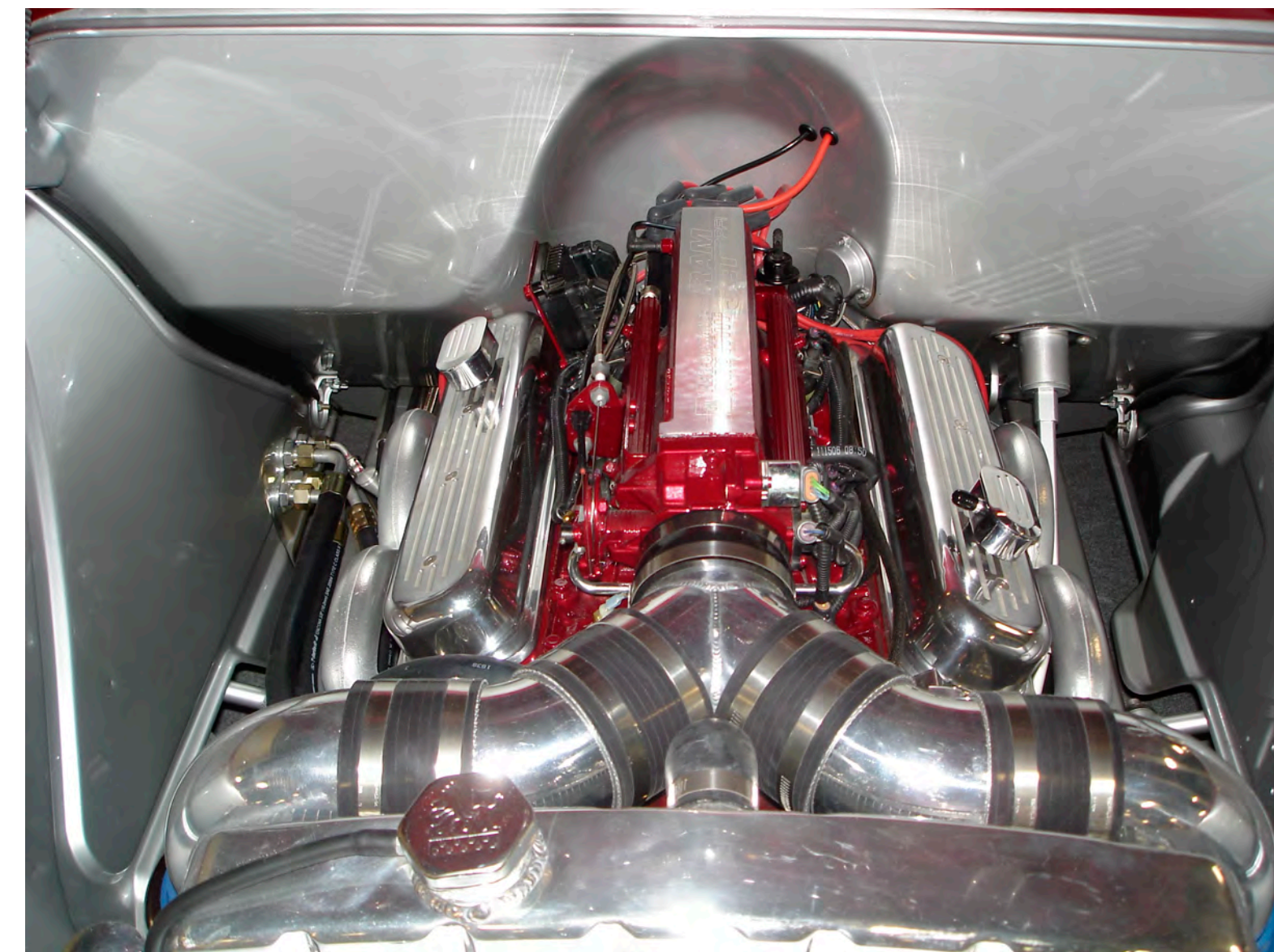
Brand new Chevy "RamJet 350" with fuel injection designed by Chevrolet to look like 1950's - 1960's fuel injected engines which debuted in 1957
