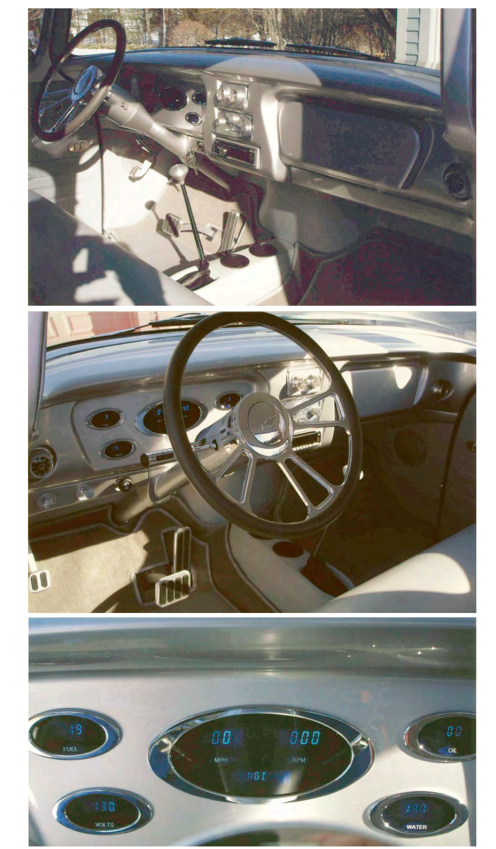
Completely re-designed custom dash with digital gauges; steering wheel has the same spoke configuration as the wheels; tilt steering column
