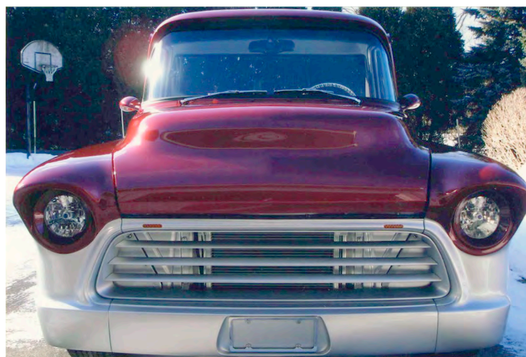
Frenched headlights; original parking lights removed; new parking/directional lights imbedded in grill; modified grill; custom rolled pan with recessed license plate; smoothed firewall
