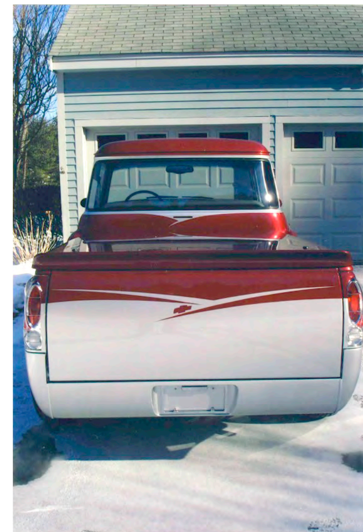
Tailgate handle moved inside; custom rolled pan with recessed license plate
