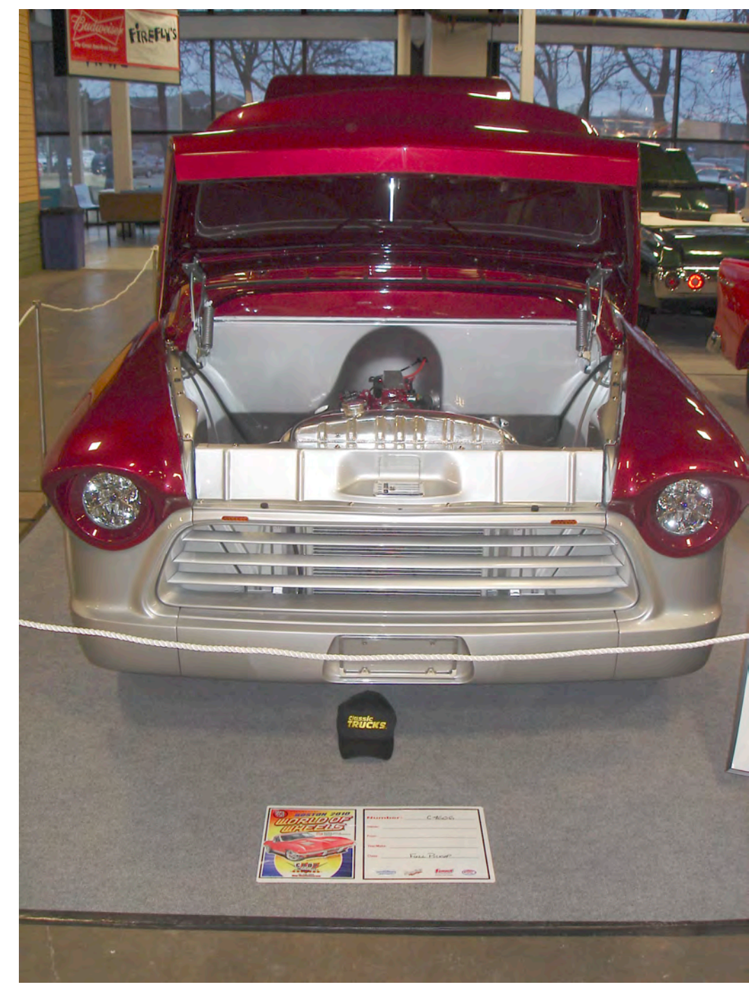
Frenched headlights; original parking lights removed; new parking/directional lights imbedded in grill; modified grill; custom rolled pan with recessed license plate; smoothed firewall
