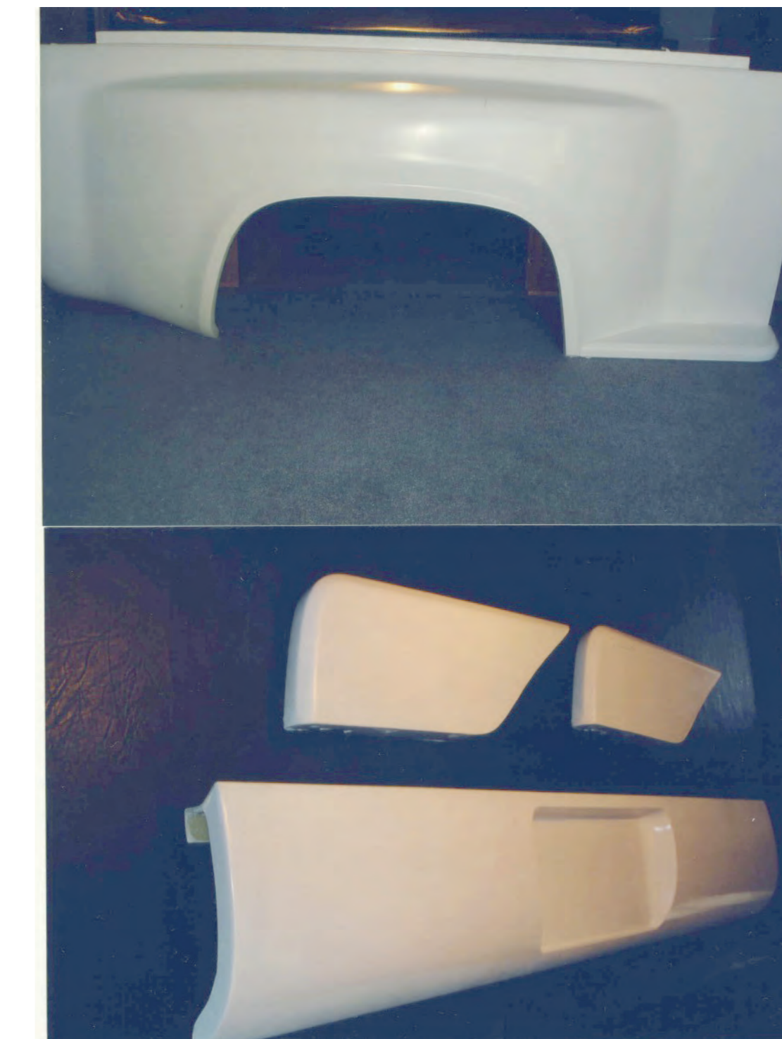
Five replicated pieces to complete fender set
